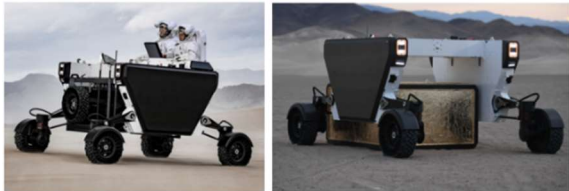
Figure 1: FLEX's modular payload interface and novel mobility system enable it to perform a multitude of functions, including crew transport, outpost logistics, robotic science, and infrastructure deployment
