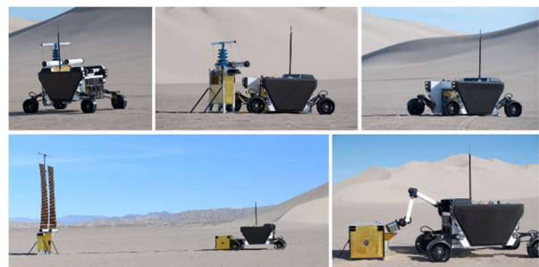
Figure 3: Astrolab recently conducted an end-to-end ISRU plant deployment demonstration at an analog test location in California
